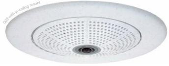
The In-Ceiling set allows mounting the cameras in suspended ceilings, for example. This type of installation provides optimum protection for the camera and reduces the visible profile to a minimum since the camera only protrudes 24 mm (1") from the ceiling.
