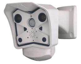
The M12 automatically selects – without high maintenance mechanical switching – either the colour sensor with daylight lens or the monochrome sensor with infrared lens for good real-colour presentation during the day or high sensitivity at night.
