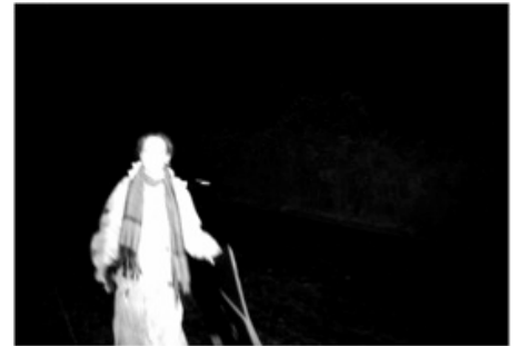
Figure 5 • Using IR illumination, objects become oversaturated very quickly.
