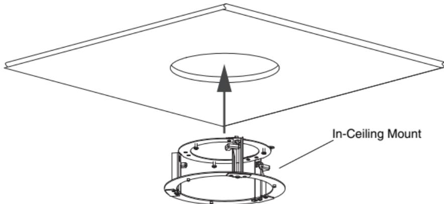
4. Tighten the three clamping screws until the mount is secured to the ceiling.
