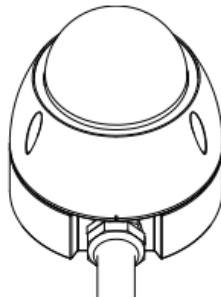
4. Mount the base on the ceiling/wall using the supplied screws and anchors. Use the supplied rubber washers to create a water tight seal between the screws and the base.
