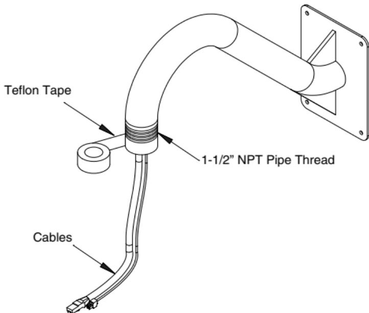
2. Screw the pendant mount onto the wall or ceiling mounting bracket until tight.
