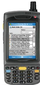
Handheld, wireless bar code scanner for viewing, creating, and instantly synchronizing changes on the go. Based on Motorola® MC75 hardware.
