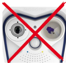
M15 with one transport plug: No operation allowed!
