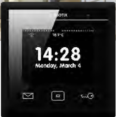
Screen saver: time, date, room temperature
