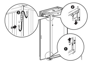
4. Remove and reinstall the latch and washer oriented as shown using a Torx T30/#2 Phillips wrench. The washer is rotated 90 degrees from its original orientation, and the latch is rotated 180 degrees.
