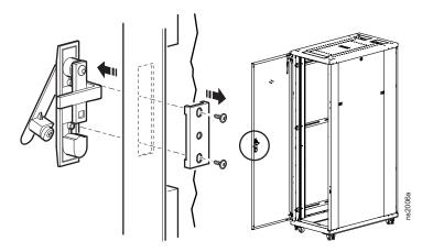
2. Unfasten the ground wire from the cabinet and door, then remove the door.
