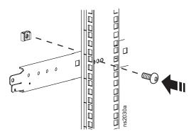
2. Move the mounting flange to the desired location and reinstall the T30 fastener at the top, middle and bottom to secure the vertical mounting flange.
