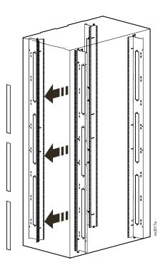
Route, secure, and organize cables using the multiple cable access openings on the cabinet roof, sides, and bottom, the accessory mounting brackets included with the cabinet, plus the variety of cable management accessories available.
