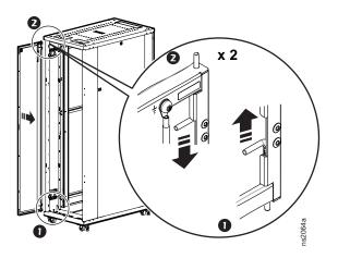
3. Connect the grounding wires.
