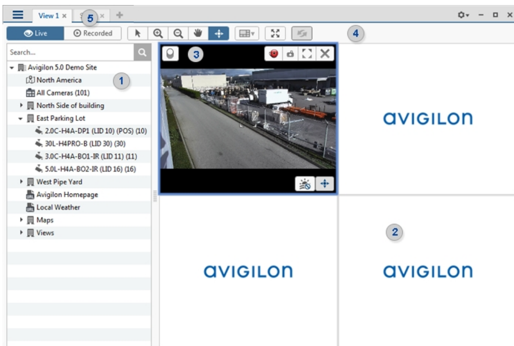
Figure 1: The Avigilon Control Center Client application window
