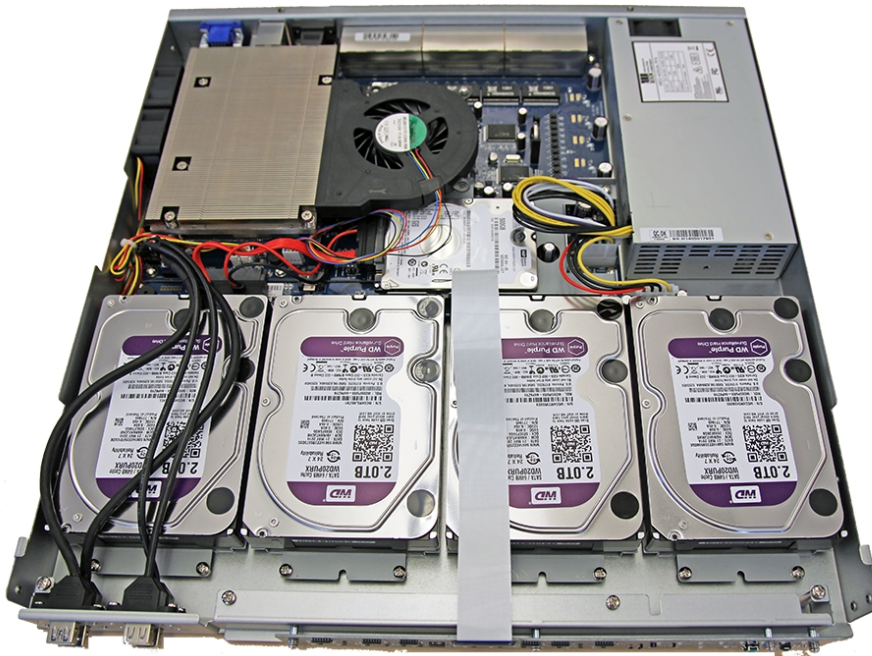
Figure 11: HD Video Appliance with the cover removed.
