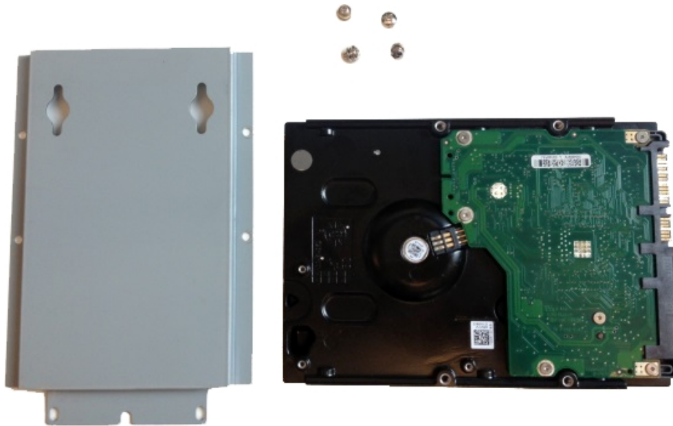
Figure 12: Hard drive removed from the base plate.
