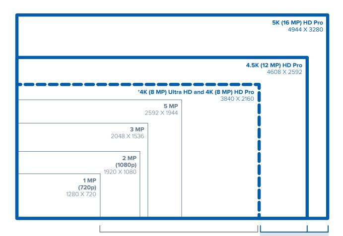
†H4 Cameras, †H4 Bullet, †H4 Dome, HD Micro Dome Cameras and HD PTZ Cameras Avigilon HD Pro Cameras 4K (8 MP), 4.5K (12 MP) and 5K (16 MP)
