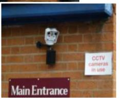
The M12 automatically selects – without high maintenance mechanical switching – either the colour sensor with daylight lens or the monochrome sensor with infrared lens for good real-colour presentation during the day or high sensitivity at night.
