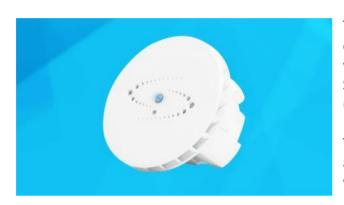
The HALO Smart Sensor is always providing vape detection with no delay in event notifications and alerts which can be received by email. Additionally, the HALO Smart Sensor can also detect tetrahydrocannabinol (THC), which is found in cannabis.
